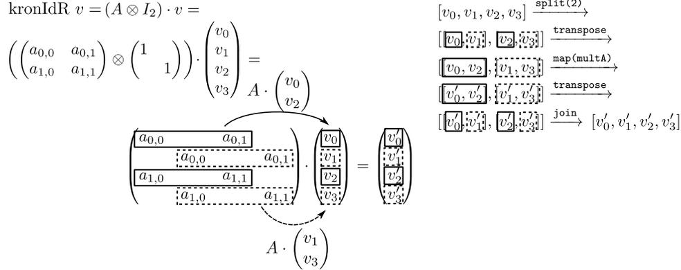
**Figure 4.** Matrix-vector multiplication of a Kronecker product with an identity matrix on the right.
