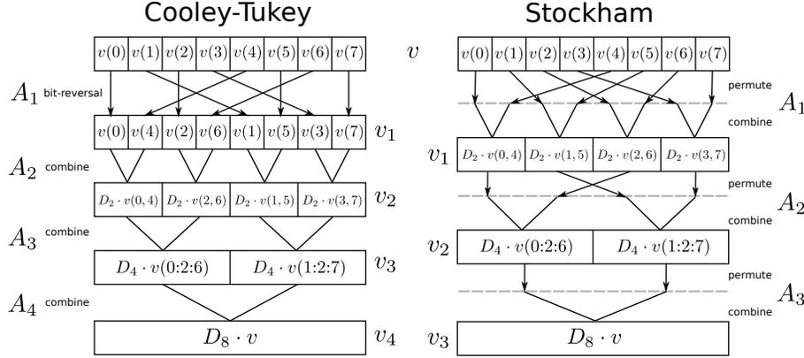
Figure 2. Example of the dataflow in the Cooley-Tukey and Stockham FFTs over an input array of size 8 (inspired by [11]).
