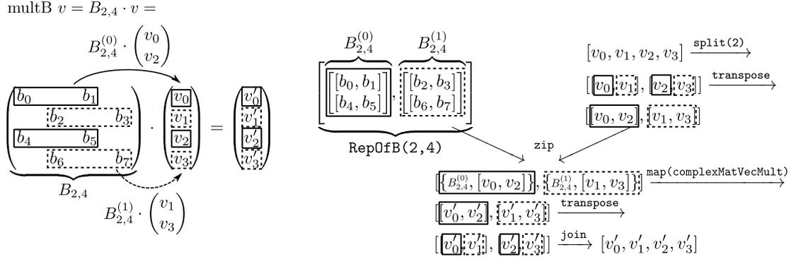
Figure 5. Multiplying a butterfly matrix with a vector.
