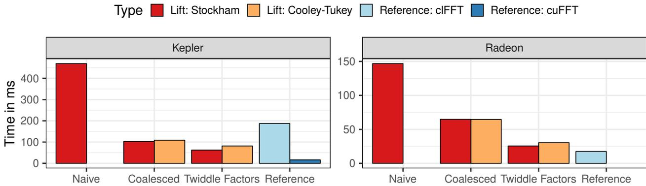
Figure 8. Runtime in milliseconds of Lift generated code (red and orange) vs. AMD’s cFFFT (light blue) and Nvidia’s cuFFT (dark blue) on Kepler K20c and Radeon RX Vega 64 GPUs.
