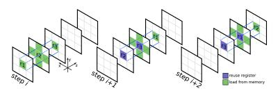
Fig. 8. A visual representation of the 2.5D tiling optimization for a single thread loading memory into registers r1, r2, and r3 which are reused over multiple iteration steps.
