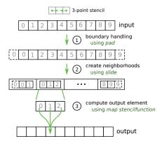
Fig. 4. Expressing a stencil in Lift using *pad* for boundary handling, *slide* for creating the neighborhood and *map* to compute the output elements. These three steps are compiled into a single OpenCL kernel by Lift.
