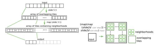
Fig. 6. Applying *slide* to the input creates tiles. Applying *slide* to tiles creates neighborhoods
