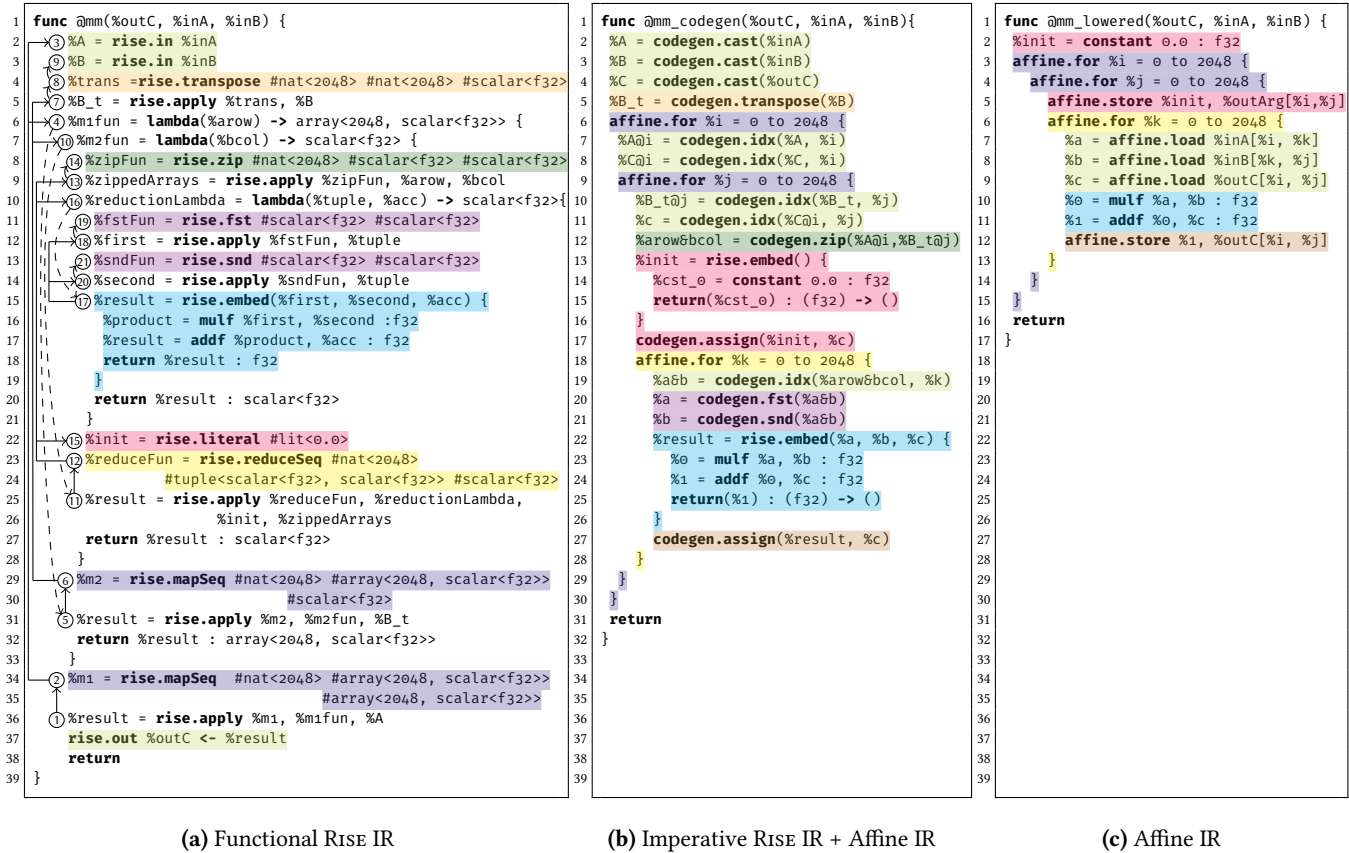
Figure 7. Lowering of matrix multiplication from RISE (left) via the intermediate imperative representation (middle) to the affine loop-based dialect (right). Colors indicate which part from the left is lowered into which part in the middle and right.
